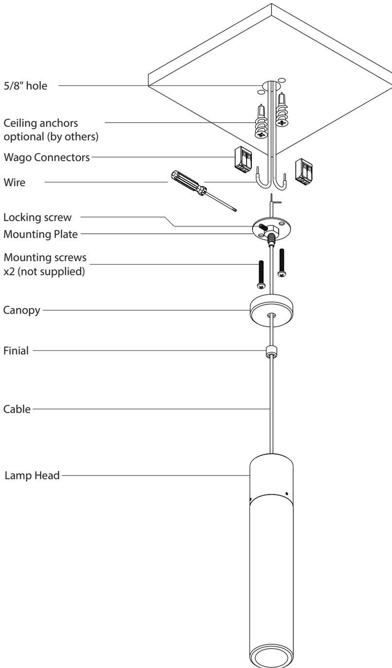
Drill 5/8" hole in the ceiling and bring class 2 supply wires (from remote driver) through the hole.
