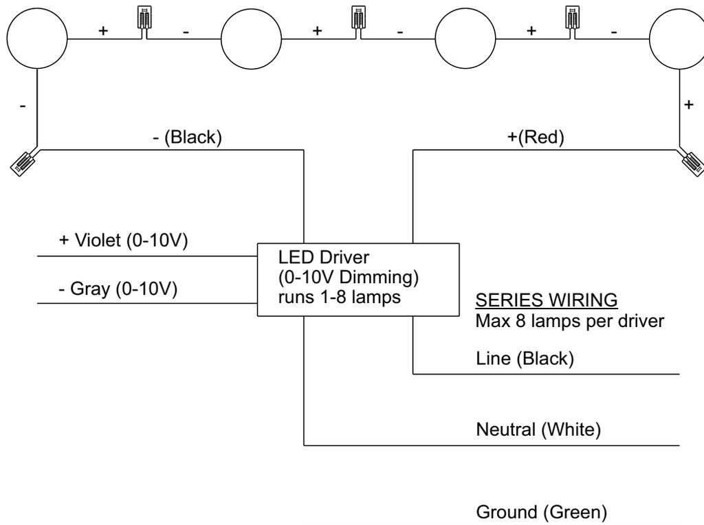
**WARNING** To be installed by qualified electrician. Power must be off when work is done. Failure to do so will cause permanent LED damage and will void warranty. Class 2 connection only. Use with Archilume constant current power supply only.
